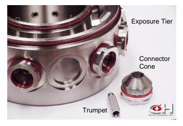
Figure 1. Partial View of Exposure Tier Showing Trumpet and Connector Cone
