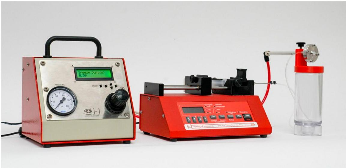
Figure 2: Syringe Fed Cough/Sneeze Mode
