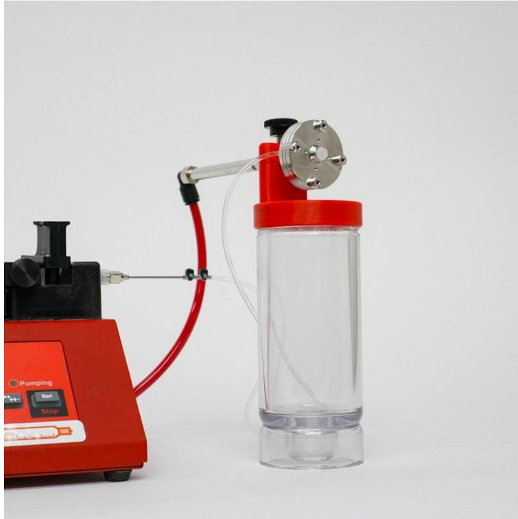
Figure 5: Syringe Fed Cough/Sneeze Mode Close Up
