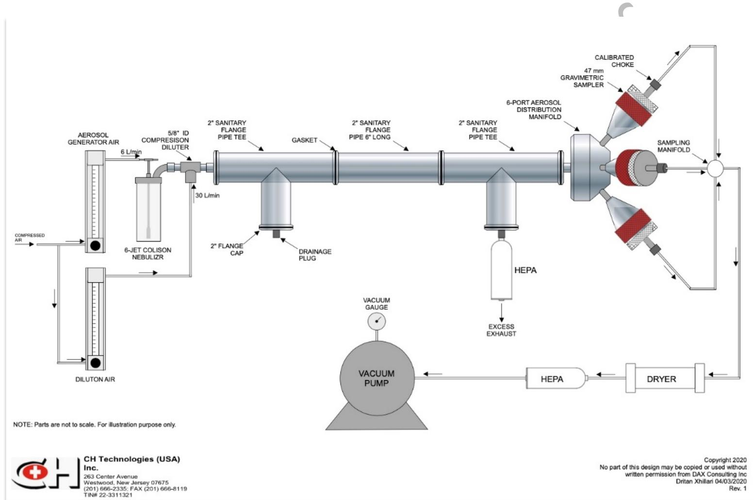
**Setup 2: Alternative to ASTM 2299: Tests with Salts or Pedialyte**
